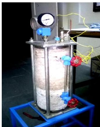
Fig 3.1 Fabrication of Steam Generator
