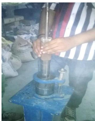
Fig.6: Compaction of Mix by Marshall Hammer
