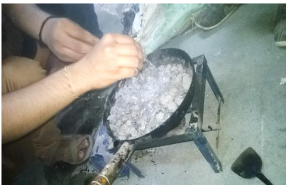
Fig.5: Heating & Plastic Coating Aggregates
