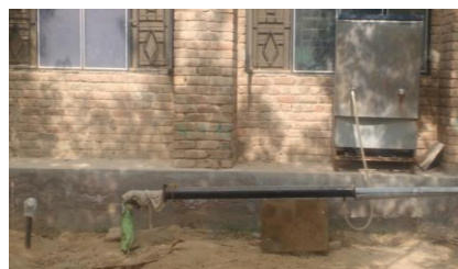
Fig. 5 Experimental Setup of Hybrid EATHE in Series Connection Coupled with Water Cooled Heat Exchanger
