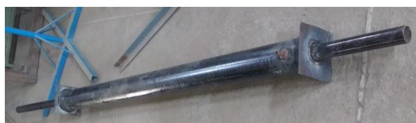
Fig. 3 Water Cooled Heat Exchanger
