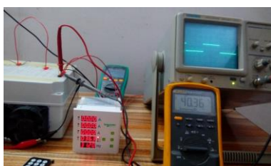
Figure 8: Pure waveform with frequency 31.2HZ and 40.36v
