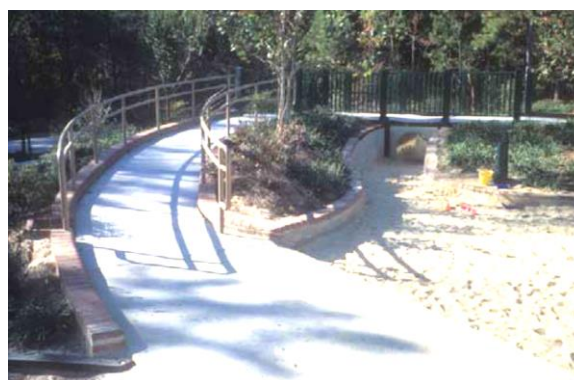
Fig. 3 Rramp over a sand play area becomes a feature in itself in this universally designed children's play area
