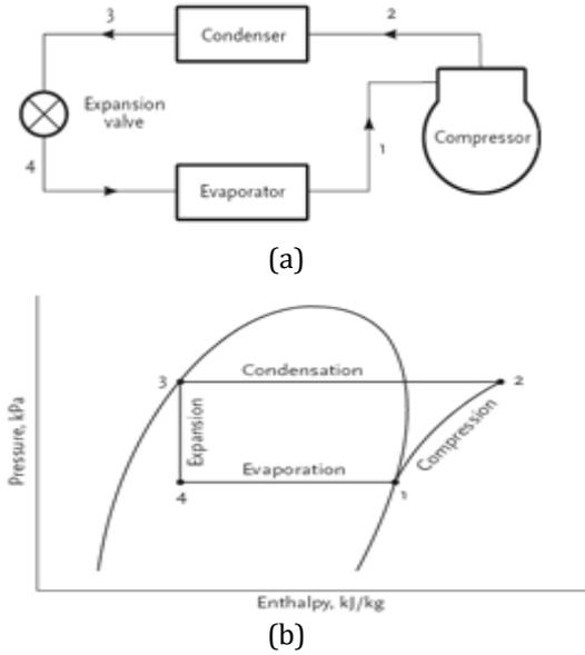
**Fig.1** (a) schematic of a simple VCRC, (b) representation on P-h scale
