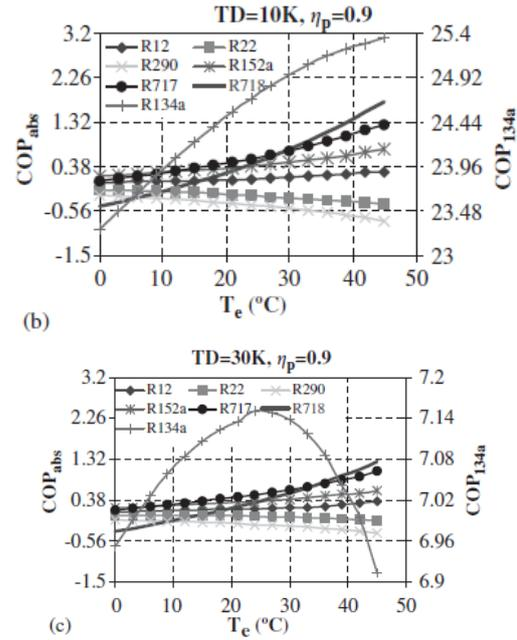
**Fig 2**  $COP_{abs}$  as a function of evaporator temperature for different TD values
