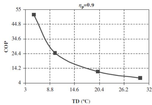
**Fig.3** COP of R718 as a function of temperature lift representative for 0...45°C. [Ali Kilicarslan *et al.*]
