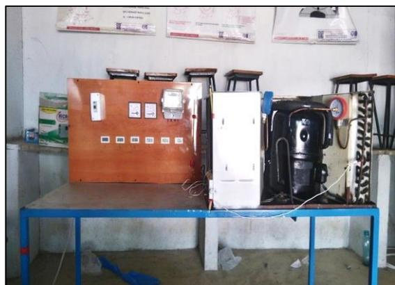
Fig. 5 Window Air Conditioner Test rig
