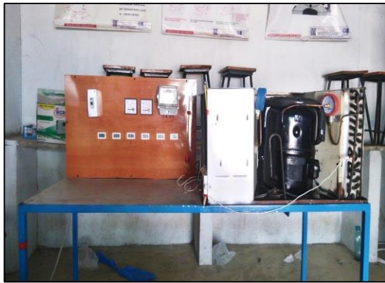
Fig. 5 Window Air Conditioner Test rig
