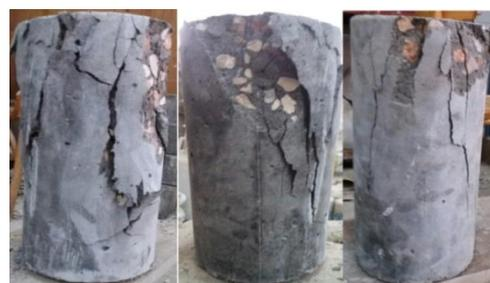
Fig.15 Shape of Failure for Tested Cylinders after the Modulus of Elasticity Test
