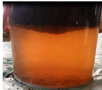
Fig.4 Shape of Rubber after Treatment with 15% NaOH
