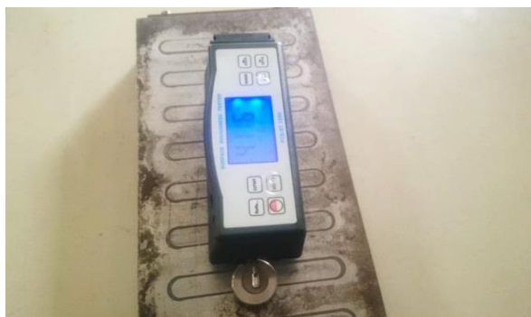
Figure 8 Measure the surface Roughness of Sample
