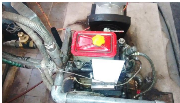
Fig.3 Installation of Magnetizer Set Up on the fuel line
