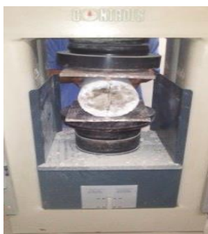
Figure 3: Split Tensile Test of Concrete Cylinders
