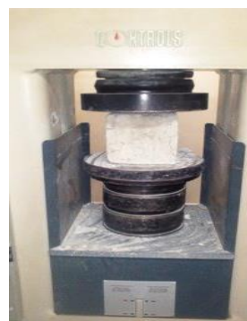
Figure 2: Compression Test of Concrete Cubes
