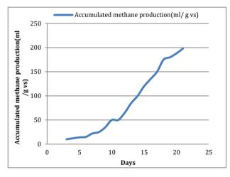
Figure 2: Accumulated methane produced from digester 1
