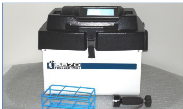
Fig 1.2 Solenoid operated Cryogenic grinder(Freezer milling)
