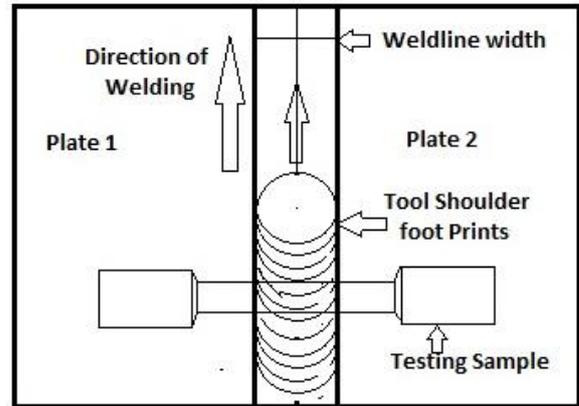
**Figure 3:** Arrangement of FSW Process
