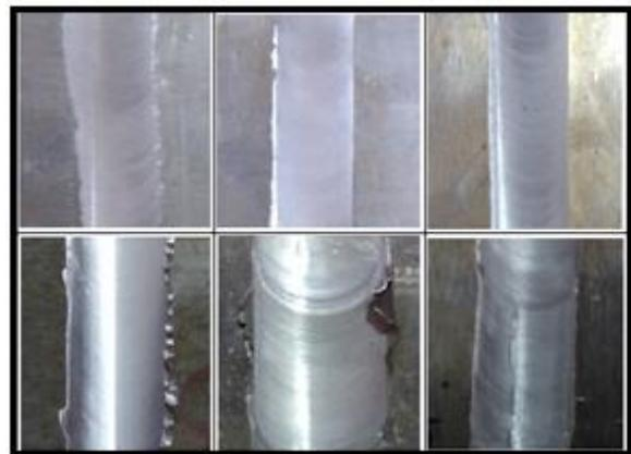
**Figure 4:** Best FSW welded joints
