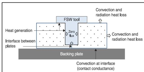
**Figure 2:** Schematic heat generation and heat dissipation diagram (Givi 2014)
