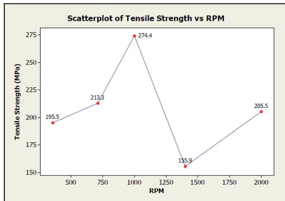
**Figure 5:** Scatter plot of Tensile Strength vs Tool Rotational Speed (RPM)
