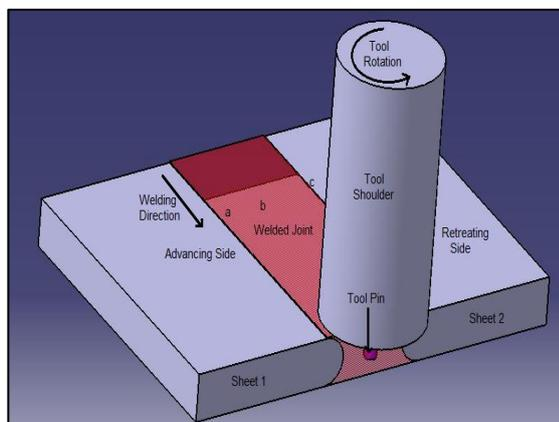
Figure 1: FSW set-up
