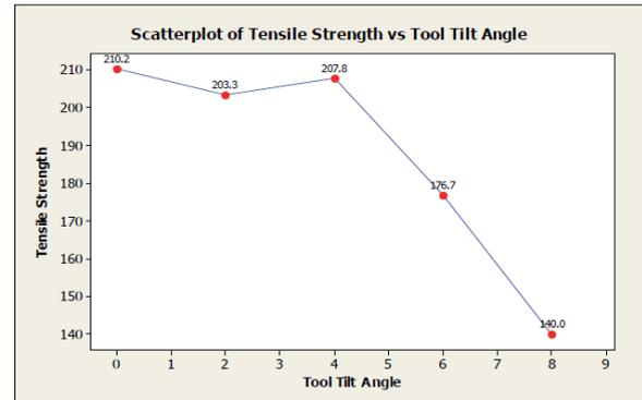
**Figure 6:** Scatter plot of Tensile Strength vs Tool Tilt Angle
