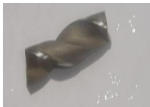
Fig. 5 Test specimen for surface and core hardness test
