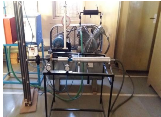
Fig Test rig of flow control valve in pneumatics
