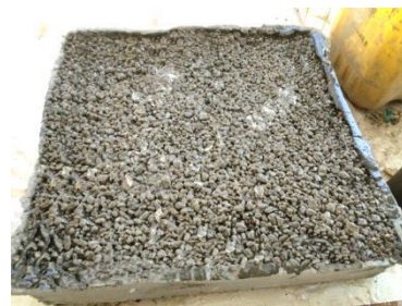
Figure 4: Final Shape of Polymer Slab Specimen
