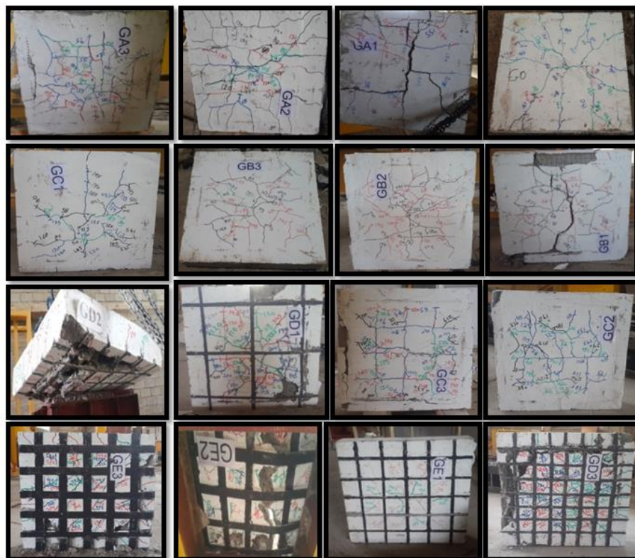
Plate 1: Slab specimens after failure
