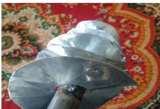
Fig.2 Auger type feed screw proto-type.
