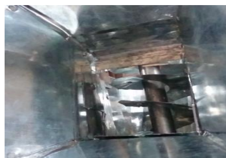
Fig.4 Auger type feed screw in casing proto-type
