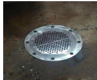
Figure 9 Tube sheet Fabrication
