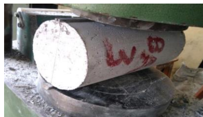
Fig. 3 Test setup for splitting tensile test
