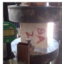
Fig.2 Test setup for compression test
