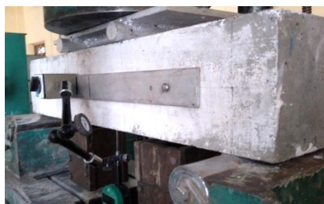
Fig. 4 Test setup for flexural test
