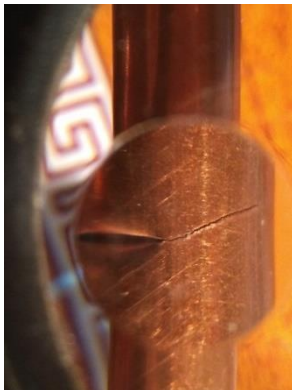
Fig.4 Illustrates a sample of crack path due to multiaxial load
