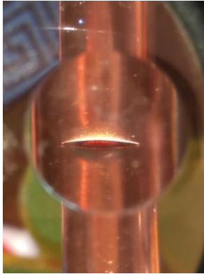
Fig.3 Initial crack in pipes (before test commencement)
