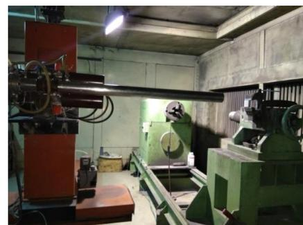
Figure 1 Detonation gun used for Spraying
