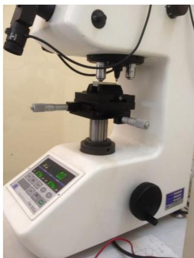
**Figure 3** Micro Vickers Used for Testing
