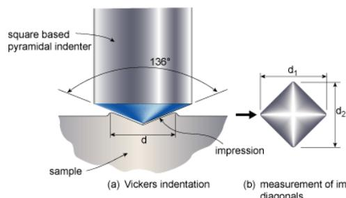
**Figure 2** Diagram representing Vickers indentation and diagonal lengths
