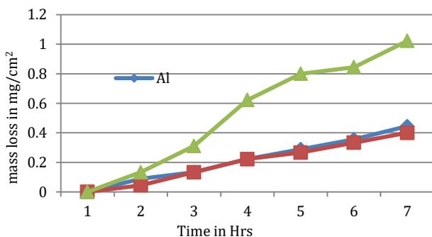
**Figure 6** Variation in Mass Loss of Al, Al<sub>2</sub>O<sub>3</sub> and Al<sub>2</sub>O<sub>3</sub>+TiO<sub>2</sub> in 35-38% HCl
