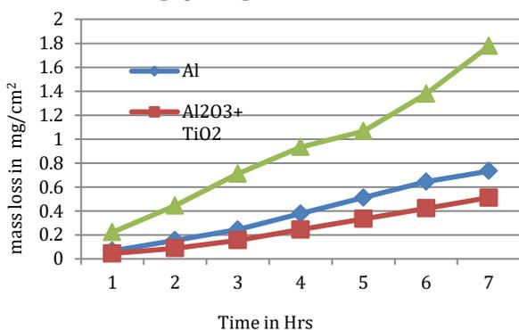
**Figure 7** Variation in Mass Loss of Al, Al<sub>2</sub>O<sub>3</sub> and Al<sub>2</sub>O<sub>3</sub>+TiO<sub>2</sub> in 35-38% HCl
