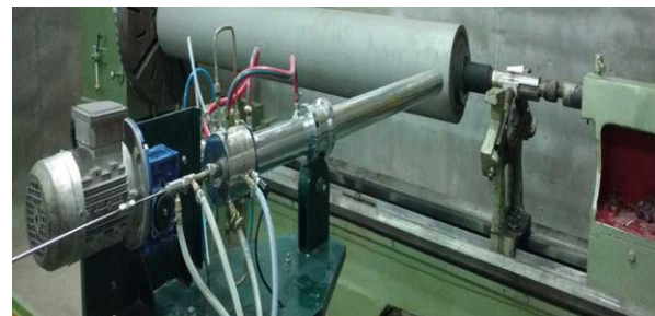
Figure 1 Detonation Gun Spraying
