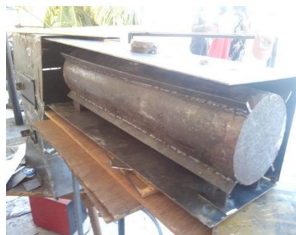
Figure 4 Evaporator tube in ducting
