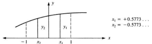
**Fig.7** Gaussian quadrature using two sampling point
