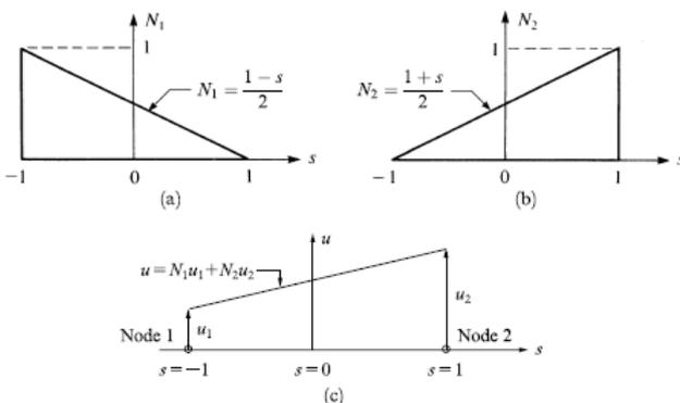
Fig.5 Shape function variations with natural coordinates: (a) N1, (b) N2, and (c) linear displacement field u plotted over element length (Daryil Logan 2007).
