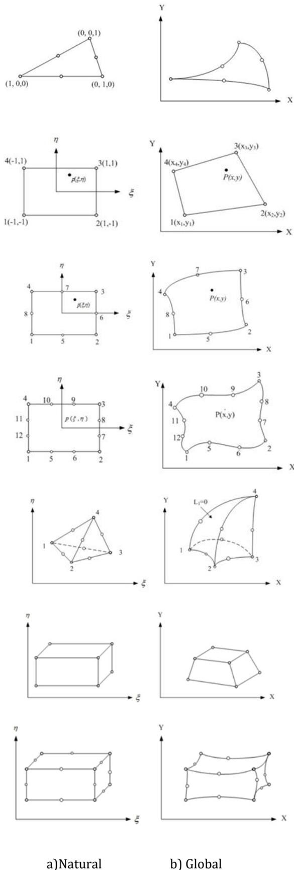
**Fig.2** Parent Elements in Natural co-ordinates and mapping in Global Co-ordinate system
