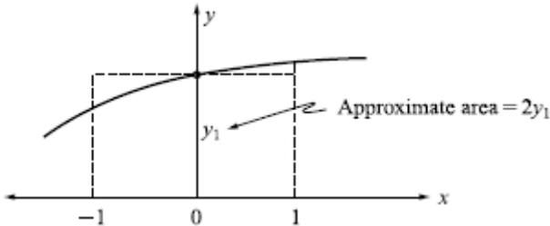
**Fig.6** Gaussian quadrature using one sampling point
