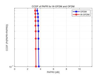
Fig. 3. PAPR of W-OFDM and OFDM with 16-PSK modulation techniques
