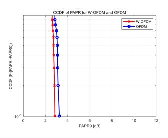
Fig. 2. PAPR of W-OFDM and OFDM with 16-QAM modulation techniques
