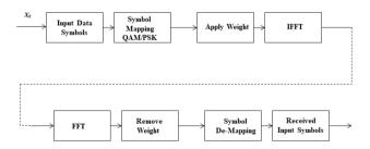
Fig-1. Block diagram of Weighted OFDM System
