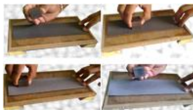
Fig.2.10 Steps for paper polishing
