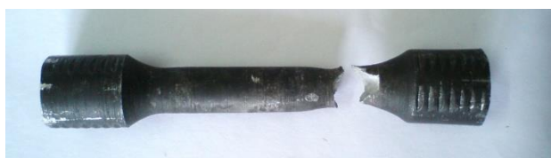
Fig.3.2 Fractured Tensile Specimen
