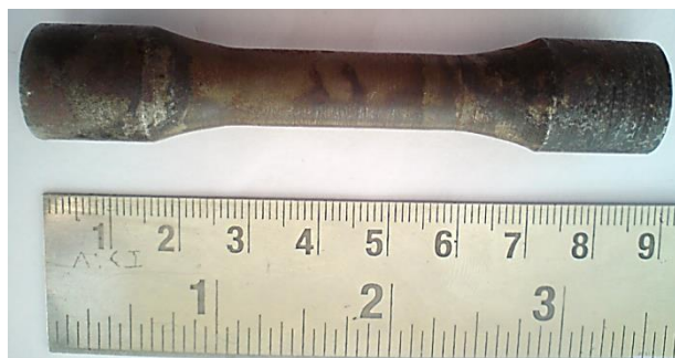
Fig.2.7 Inter-critical specimens at 750 °C
