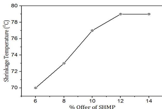
**Fig.2** Effect of SHMP dosages on the Ts of wet white leather (Tanning time = 2 hour, pH of the bath = 3)
