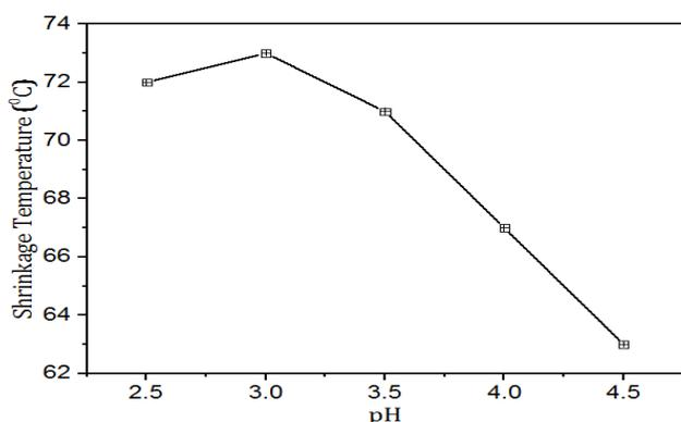
**Fig.1** Effect of pH on the Ts of wet white leather (Tanning time = 2 hour, dose of SHMP = 8% of pelt weight)
