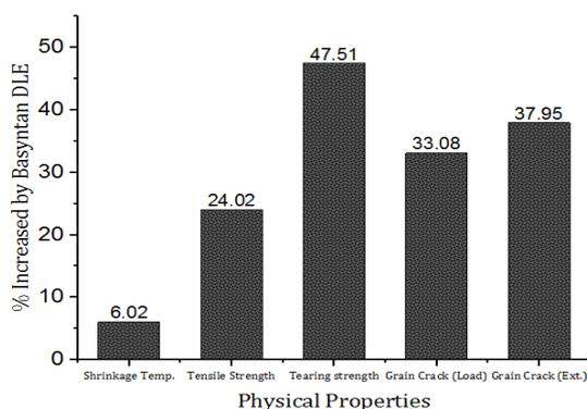
**Fig.2** percentage enhancement of different physical properties of wet white leather by Bsyntan DLE assisted SHMP tanning
