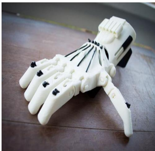
Fig.7 Overall Design of EMG Prosthetic Arm
