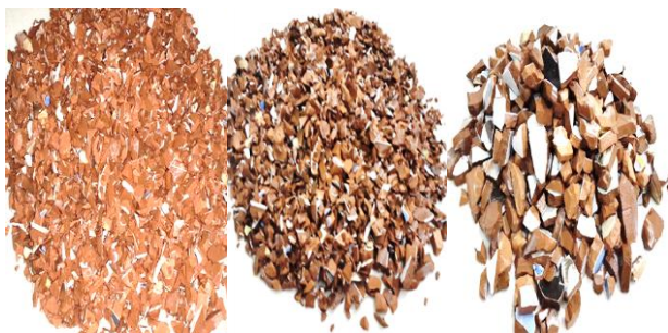
Fig. 8 Photos of Graded Ceramic Media used
