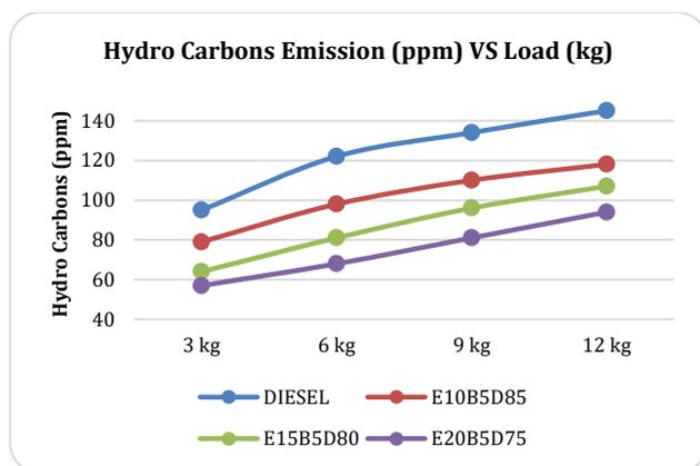
**Figure 6** Variation of Hydro Carbons Emission with Load
