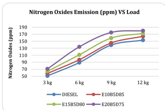
**Figure 7** Variation of Nitrogen Oxides Emission with Load
