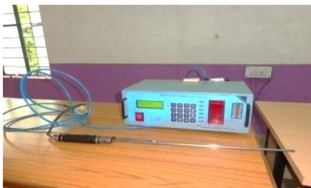
Figure 2 Exhaust gas analyser
