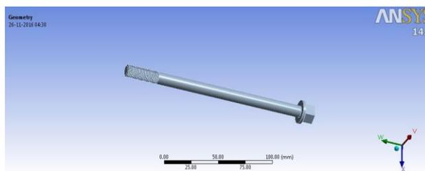
Fig.2.1 Geometry of the bolt in ANSYS
