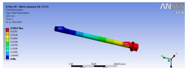
Fig.3.1. Total deformation of engine head bolt
