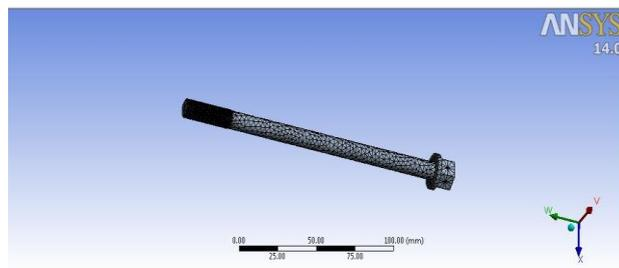
Fig.2.2 Meshed model of engine head bolt
