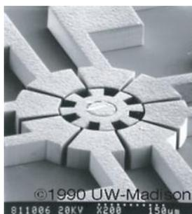
**Figure 1** SEM image of an electrostatic micro-motor with eight rotor and 12 stator poles
