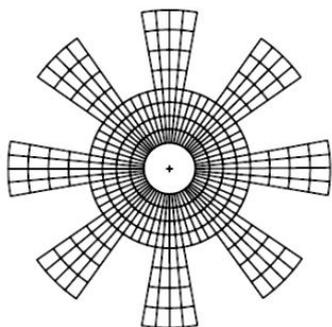
**Figure 3** Finite element mesh using 2D, four nodal shell elements
