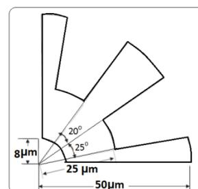
**Figure 2** Plan view (2D) of a quarter of micro-motor rotor
