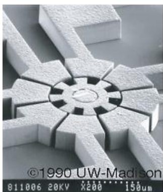
Figure 1 SEM image of an electrostatic micro-motor with eight rotor and 12 stator poles
