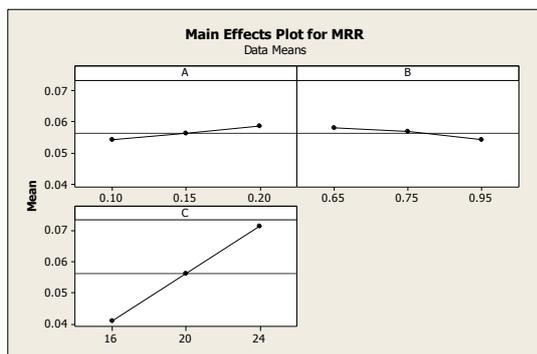
**Fig. 1** Main Effects Plot for M.R.R of TiC
