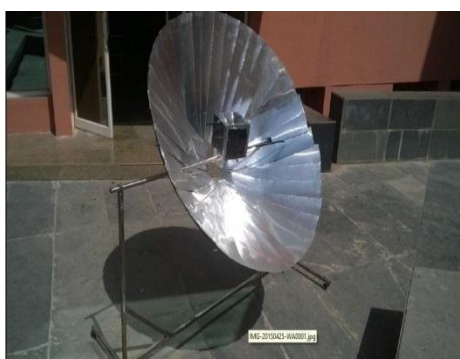
Fig.7 Experimental setup of solar water heater
