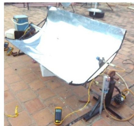
Fig.2. Cylindrical Parabolic Trough Collector
