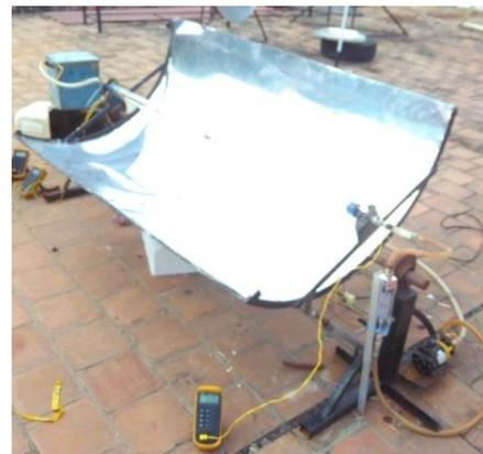
Fig.2. Cylindrical Parabolic Trough Collector
