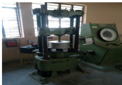
Fig.11 Hot Extrusion Setup
