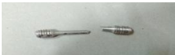
Fig.16 Tensile testing break specimen
