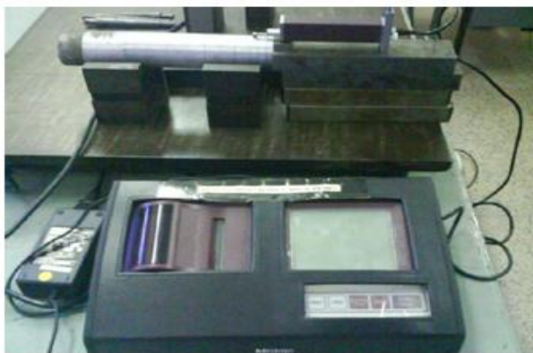
Fig.3 Photographic view of stylus during surface roughness measurement
