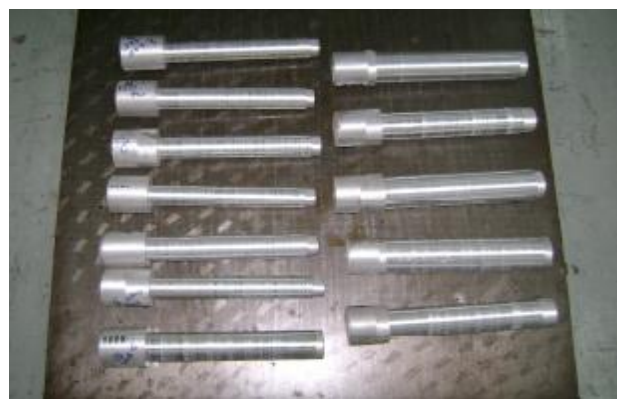
Fig.1 Al-SiC p composite samples used as work pieces (50 mm dia. and 300 mm long)
