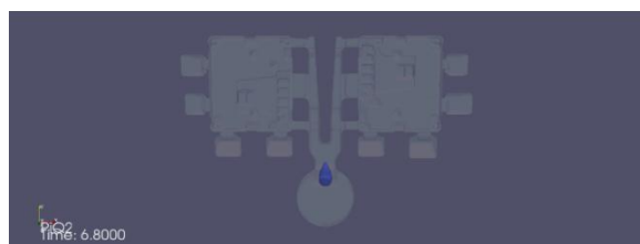
Fig.6 Heat Sink Mold Flow Analysis (Solidifying Time=6.8 sec)
