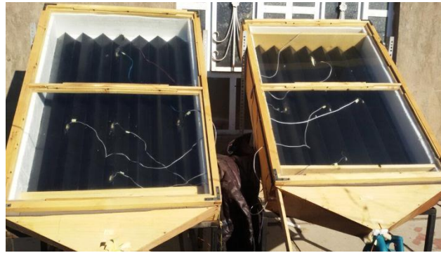
Fig. 1 Photograph of two solar air heaters
