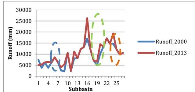
Fig.11 Comparing Runoff of 2000 and 2013 in each sub-basin
