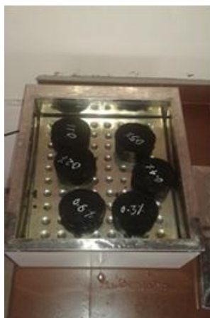
Figure 3.4: Waterbath at 60°C
