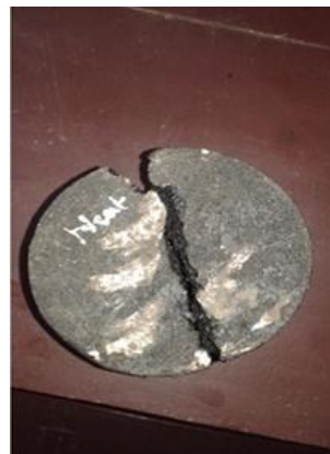
Figure 3.8: Failure of Specimen after IDT Test
