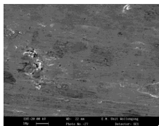
Fig. 3 SEM micrograph of worn surface tested at a load of 2 kg for NIS 1
