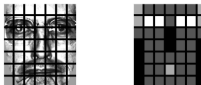
Fig.6: A facial image divided into 7 X 7 windows and the weights set for the weighted Chi square dissimilarity measure. Black squares indicate weight 0.0, dark gray 1.0, light gray 2.0, and white 4.0.
