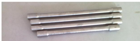
Fig. 2. Specimen used for tensile testing
