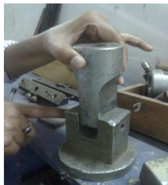
Fig. 4. Jig Used For Shear Test
