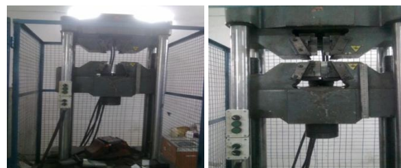
Fig. 1. 50 Ton Universal Testing Machine
