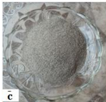
Figure 1 (a) Rice Husk (RH); (b) RHA burned at 700 °C; (c) RHA heat treated at 1100 °C for 2 hrs
