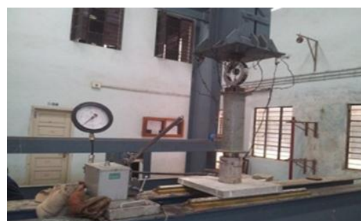
Plate 6: Test setup for Flexural strength Of Prisms
