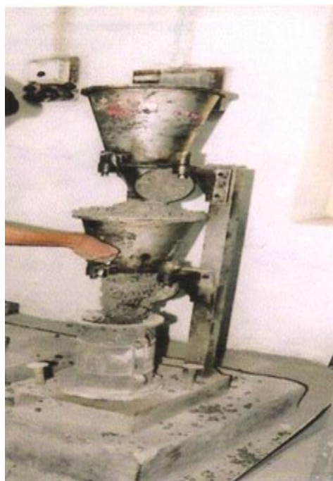
Plate 3: Compaction factor test
