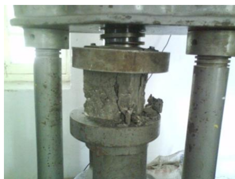
Plate 5: Test set up for Cube Compressive Strength
