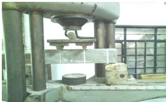
Plate 8: Test setup for Flexural Fatigue Strength
