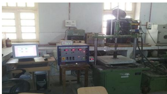
Plate 7: Test setup for Static Point Load of Slabs
