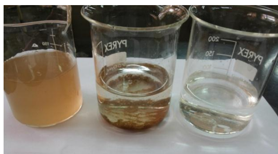
Figure 3 produced water initially and after adding coagulant and flocculent materials
